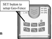
Press the SET button to set a 200 m Geo-fence around the device.
